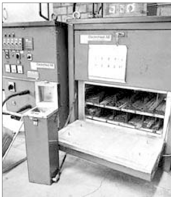
Dry cabinet for storage of electrodes.
