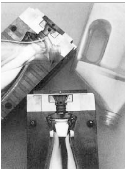
Two halves of a MOLDMAX HH beryllium copper blow mould.
